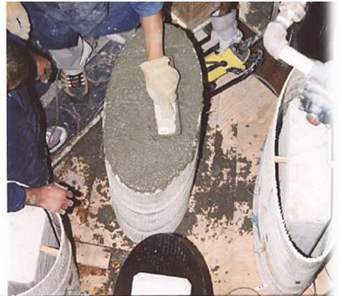
Figure 3.7(d) Casting of expansive cement concrete (4 th step)
