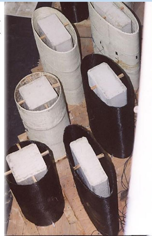
Figure 3.7(d) Casting of expansive cement concrete (4 th step)
