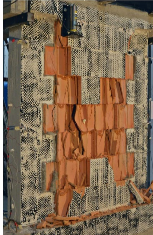
Failure of the wall
